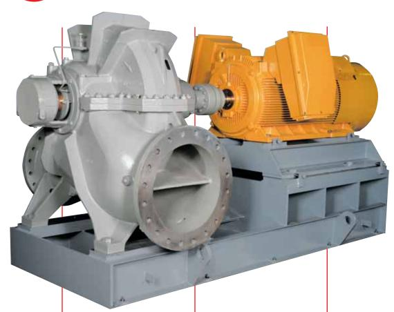
Bearing Housings with 360° attachment and unique fastening to upper and lower casings provide superior bearing stability and shaft support. Perfect shaft alignment is assured by a full register fit to the casing. Bearing housings and stuffing boxes can be easily removed and reinstalled.
